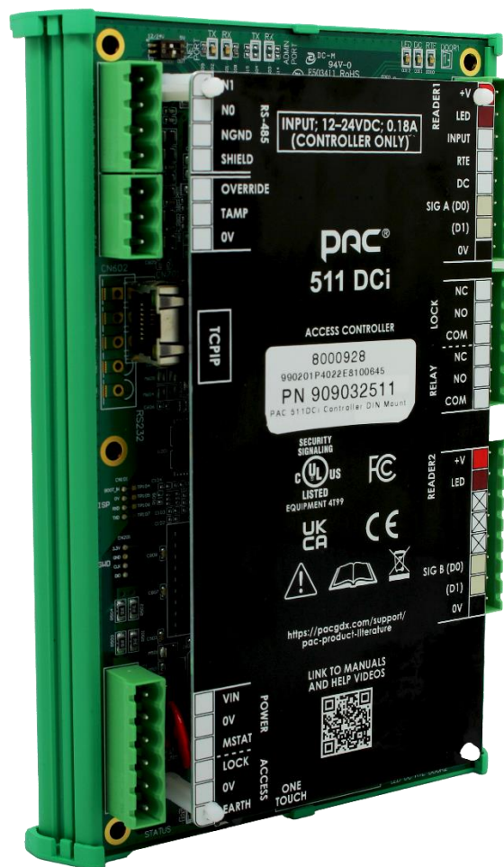
Figure 6 - PAC 511 DCi Controller
