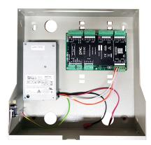
Complete with lockable metal case, tamper switch and 3 Amp PSU
